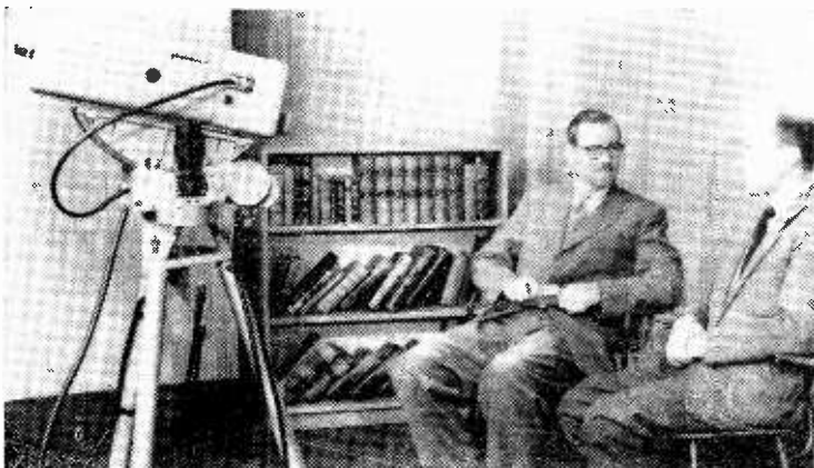
REMOTELY CONTROLLED television camera developed by the B.B.C. Engineering Division is being used experimentally at one of the interviewing studios near Broadcasting House. All its functions—pan, tilt, focus, zoom and iris—are operated by servo-motors controlled from the news studio at Alexandra Palace, about six miles away. The camera is also controllable by the interviewer, who, as seen in this photograph, holds a small push-button control box.
